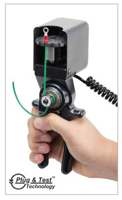
The MR06-200 wire crimp pull sensor is a hand-operated solution for measuring wire crimp pull-off forces. The ergonomic handles and convenient tensioning mechanism make field measurements a breeze for applications up to 200 lbF (1,000 N). Squeeze the handles together to increase tension on the sample until a break occurs. The peak force is recorded by the indicator.
