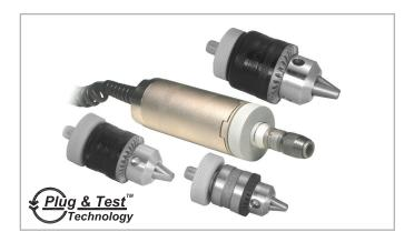
Series R51 smart sensors measure bi-directional torque for numerous applications across virtually all industries. Interchangeable Jacobs chucks and bit holder add flexibility for a variety of applications. The sensors can be used as hand held devices or mounted to a test stand. Superb overload protection adds peace of mind. Capacities available from 10 ozFin to 100 lbFin [7 to 1150 Ncm]. Compatible with Mark-10 indicators (sold separately) through unique Plug & Test™ technology.
