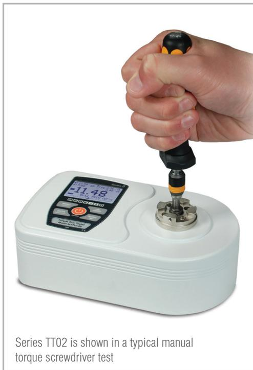
Series TT02 is shown in a typical manual torque screwdriver test
